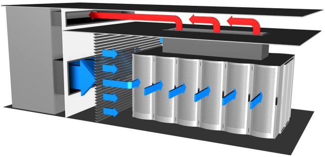
Innovative flooded room cooling, utilising hot aisle containment allowing up to 80kW per rack
